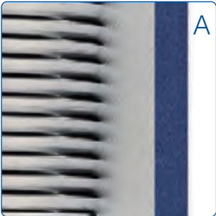
Zigzag thread Lead=8T.P.I Taper=1:16
