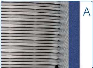
API Buttress Thread
