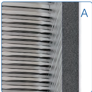
Hooked Thread Taper=1:16 TBG: 2-3/8in~2-7/8in: (8T.P.I.) 3-1/2in~4-1/2in: (6T.P.I.) CSG: 5in~8-5/8in: (5T.P.I.) 9-5/8in~20in (4T.P.I.)
