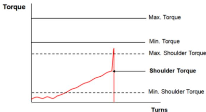
**Minimum specified torque is not obtained. Break out and evaluate.**
