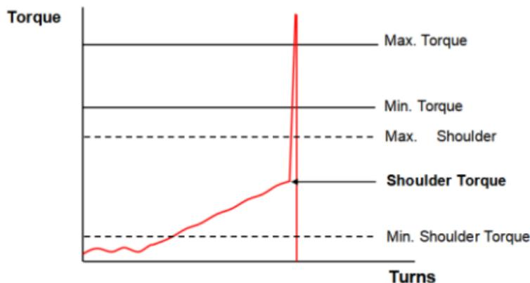
**Maximum specified torque is exceeded. Break out and evaluate.**
