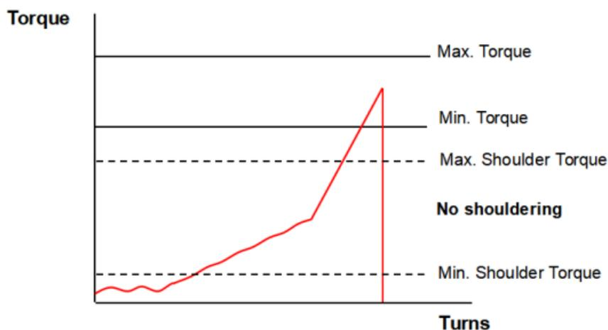
**Torque shoulder does not engage. Break out and evaluate**
