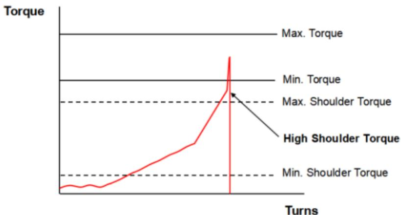
**Shoulder torque is outside the specified shoulder torque window.**
